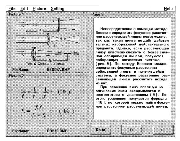
Fig. 4.One page of GuideShell-program: Bessel method for Focal Leight Determination (Single Lenses and Lenses Sistems)
