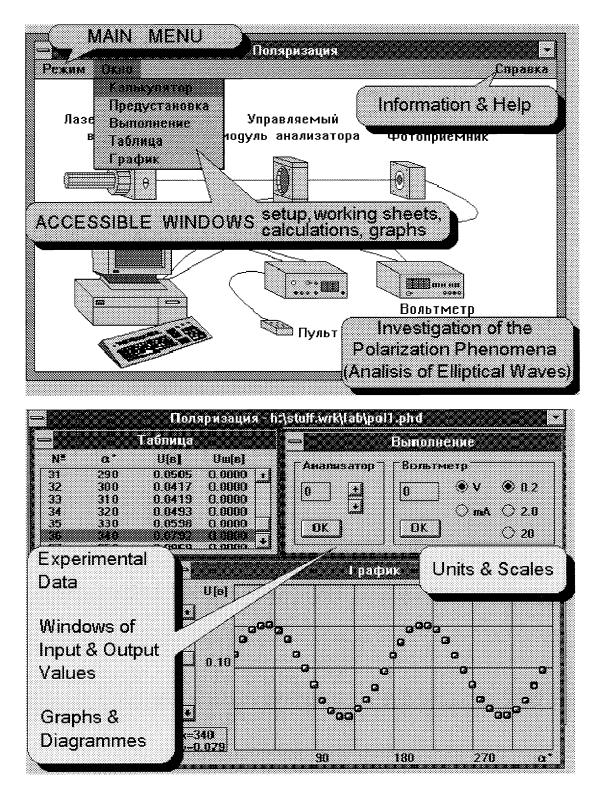
Fig. 3 View of the Screen (above) and Working Sheet (below) of LabShell programm for studying Polarization Phenomena by using Laser Beam and different phase Objects
