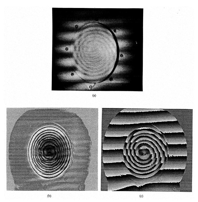
Figure 5. Phase Stepping Technique a) Real-time Hologram b) Vibrational Fringes c) Static Deformation Fringes.
