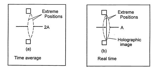
Figure 3. Recorded Diaphragm Displacement a) Time Average Holography b) Real Time Holography
