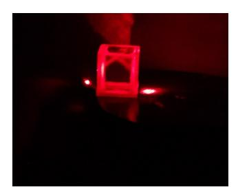
Total Internal Reflection of laser light in water
