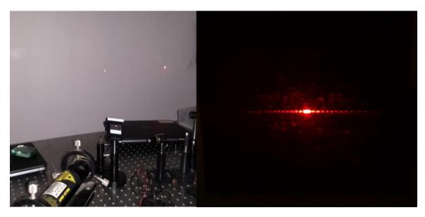
Diffraction of laser through diffraction grating.
