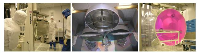
Figure 8. Optics Support Facility. (Left) Handling of a truncated 94 cm fold mirror. (Middle) Interior of the coating chamber during the coating of a truncated 94 cm fold mirror. (Right) Final product for a 75 cm HR coating (200 lb weight).
