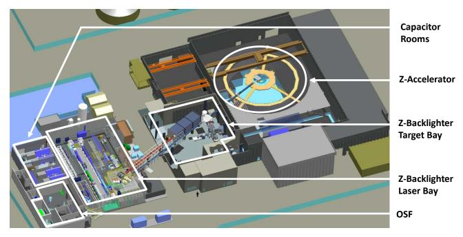
Figure 2. A bird's eye view of the Z-Accelerator and the Z-backlighter Facility. The Z-backlighter is made up of about  $20,000 \text{ ft}^2 (1,800 \text{ m}^2)$  of space from the Optics Support Facility (OSF), the Laser Bay, the Target Bay, and the Capacitor Rooms (used to drive the flashlamps that pump the main Z-Beamlet and Z-Petawatt slab amplifiers). For scale, a human is shown just below the Target Bay.
