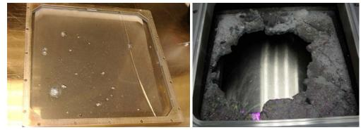
Figure 7. Used Debris Shields. (Left) Moderate damage on Z shot consisting of several shrapnel sites and "soot" coating. (Right) Severe damage during a Z shot.
