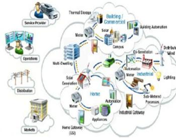
Fig. 2: Smart Grid Domain Model (Source: NIST)
