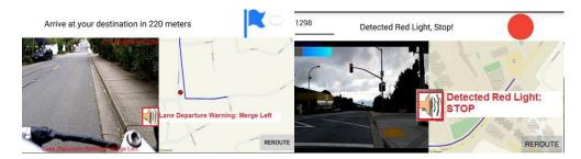
Figure 2: blindBike directs low vision person with auditory prompts for road following and intersection detection.
