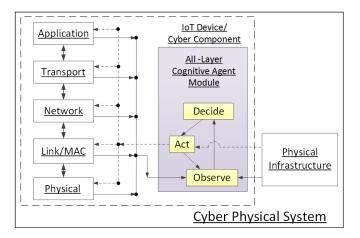
Figure 1. Block diagram of the cross-layer IoT device for cyber physical systems, where an all-layer cognitive module integrates information from the networking environment and the physical infrastructure to provide self-aware autonomous operation of the device.
