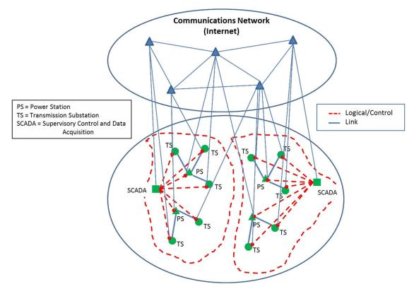
**Figure 3: Electrical Power Grid**
