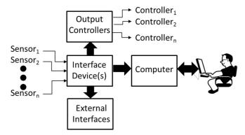
Figure 1: Overall Controller Architecture
