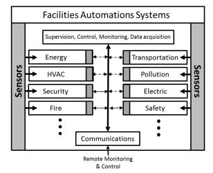
Figure 2: Examples of Industrial/Commercial Controllers
