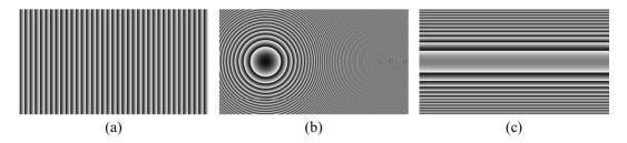
Figure 10. Special phase distribution, such as (a) Deflected plane wave phase pattern at a specific diffraction angle, (b) Mixture of spherical and deflected plane wave phase pattern, and (c) Cylindrical wave phase pattern.
