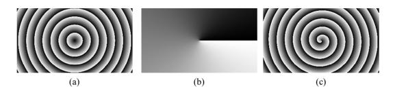
Figure 12. Special phase distribution, such as (a) Axicon phase pattern, (b) Vortex pattern, and (c) Combination of axicon and vortex phase pattern.
