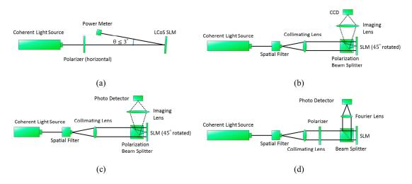
Figure 7. Experiment setup of (a) Light utilization, (b) Uniformity, (c) Response time, and (d) Diffraction efficiency.
