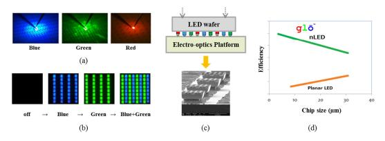
Figure 3. (a) Photo of actual nanowire LEDs, (b) The arrangement and switch method of nanowire LEDs, (c) SEM of actual nanowire chip, and (d) The efficiency vs. chip size based on gloss nanowire LEDs.
