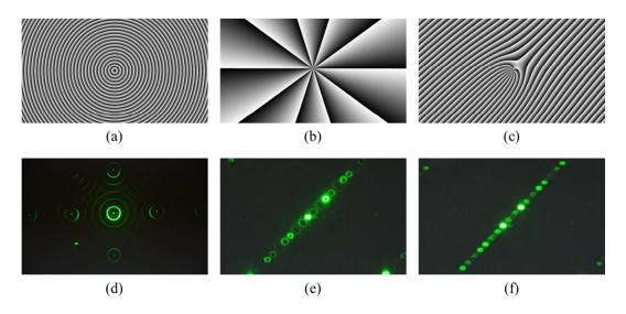
Figure 13. Diffraction image results at different axicon and vortex condition, (a) Axicon phase pattern, (b) Vortex pattern, (c) Fork pattern (vortex pattern + x & y shift pattern), (d) Diffraction image of axicon, (e) Diffraction image of fork pattern at vortex order 10, and (f) Diffraction image of fork pattern at vortex order 1.
