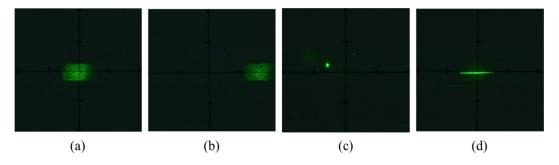
Figure 11. Various types of wavefronts on the screen, (a) Non-modulated and deflected plane wave, (b) Deflected plane wave at a specific diffraction angle, (c) Focused convergent spherical wave at a shifted angle, and (d) Convergent cylindrical wave.
