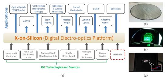
Figure 1. (a) Various application based on Digital Electro-optics Platform (X-on Silicon), (b) Digital Electro-optics Platform, (c) 3D holographic display based on LCoS-SLM, and (d) 3 color microdisplay based on µLEDoS.
