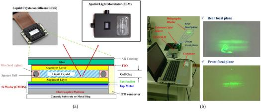
Figure 2. (a) The architecture and product photo of reflective type LCoS-SLM, and (b) Two diffraction images are demonstrated at different focal plane.
