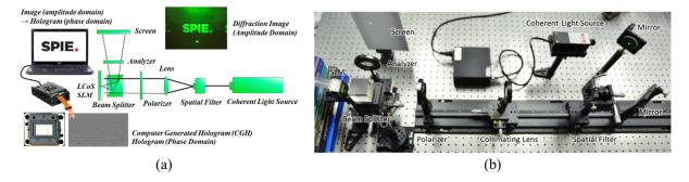
Figure 8. (a) Experiment setup and diffraction results by using CGH pattern generator and CGH modulation software, and (b) The experiment setup photo of measuring the diffractive image.
