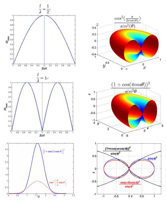
Figure 13 Half-wavelength antenna and full-wavelength antenna and their radiation patterns
