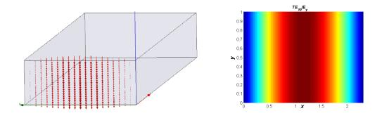
Figure 5 The distribution of electric fields for  $TE_{10}$  mode in rectangular waveguide
