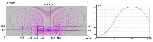
Figure 1 Magnetic field of 5 groups of solenoid
