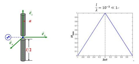
Figure 12 Sketch of short center-fed thin linear antenna and its current distribution
