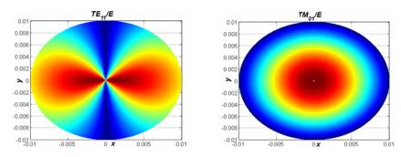
Figure 6 The distribution of electric field for TE<sub>11</sub> and TM<sub>01</sub> modes in cylindrical waveguide
