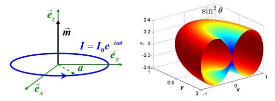
Figure 10 Circle antenna and its magnetic dipole radiation distribution
