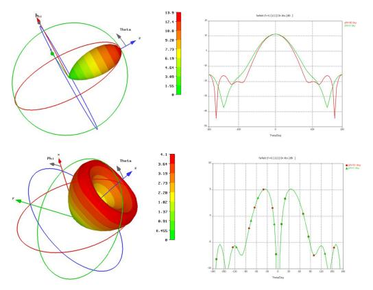
Figure 14 The 3D and 2D directional diagram for radiated (up) TE<sub>11</sub> and (down) TM<sub>01</sub> modes in space
