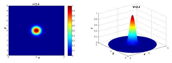
Figure 7 The 2D and 3D distributions of light intensity for  $LP_{01}$  mode in optical fiber
