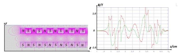
Figure 2 Partial magnetic field of periodic permanent magnets
