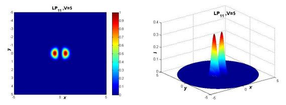
Figure 8 The 2D and 3D distributions of light intensity for LP<sub>11</sub> mode in optical fiber
