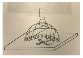
Figure 3. (a) Reflective dome lighting prototype design
