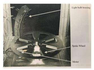
Figure 4. Rotating arc prototype for both light sources as well as uniformity testing apparatus
