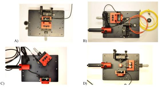
Figure 3: Examples of setups: A) Micro-camera, B) Fiber optics, C) Speckle movement sensor and D) interferometer
