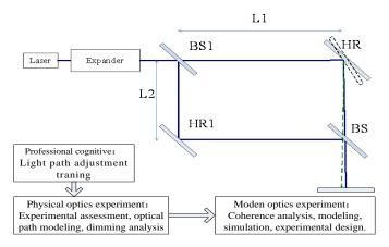
Figure 5. The progressive experiments concerning the Mach-Zehnder interferometer.
