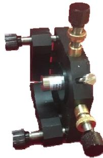
Fig. 3 a designed adjusting rack
