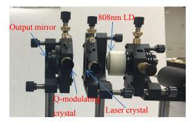
Fig. 9 Set-up diagram for Q-modulation output of 1064nm laser
