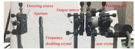
Fig. 2 Experimental system of laser-diode-pumped solid-state laser
