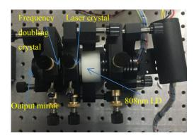
Fig. 7 Set-up diagram for observing frequency doubling effect of solid-state laser
