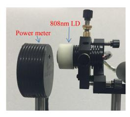
Fig. 4 Experimental installation for measuring I-P curve of laser diode
