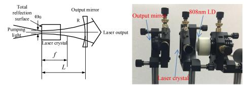
Fig. 5 Structure of resonant cavity of solid-state laser
