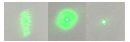
Fig. 8 Several output transverse modes of 532nm laser
