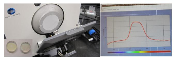
Figure 13. LEFT: Integrating sphere inside a spectrophotometer. CLC samples between two glass substrates are shown in insert. RIGHT: A selective reflection curve (spectral dependence of reflectivity) of a photonic bandgap CLC structure.
