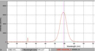
Figure 10. LEFT: Three solutions of NQDs and UV source for excitation of NQD fluorescence. RIGHT: Typical fluorescence spectrum of NQD.
