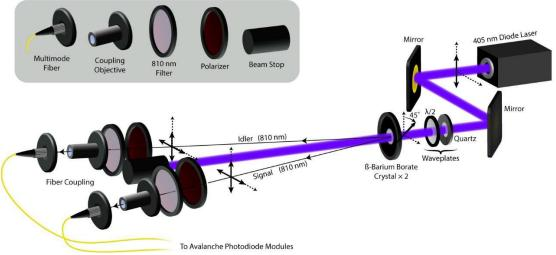
Figure 4 (prepared by R. Lopez-Rioz) shows the schematics of experimental setup of polarization entangled photons with two BBO crystals and a diode laser. We did not use a quartz plate for compensation a phase  $\Delta$  to obtain entangled photons in a last version of a setup with a 405 nm laser, although in an OPT 253 class students investigated its effect on results by its rotation around two axes.
