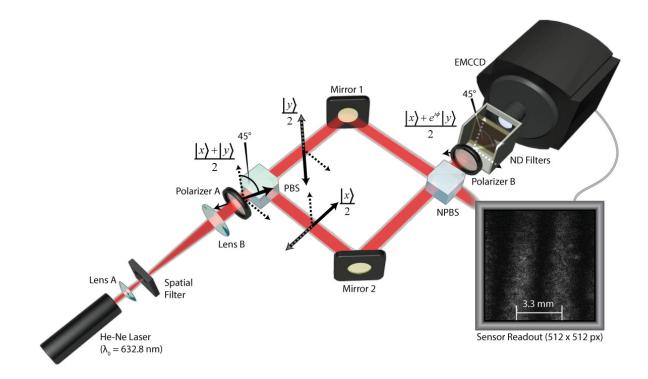
Figure 10 (prepared by R. Lopez-Rios). Setup for a Mach-Zehnder Interferometer. PBS: polarizing beam splitter; NPBS: non-polarizing beam splitter. At each point where the system state changes the polarization vector is shown.
