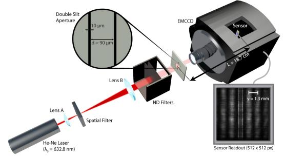
Figure 9 (prepared by R. Lopez-Rios). Setup of a single photon Young's double slit experiment. ND: Neutral density filters; EMCCD: electron multiplying CCD camera; He-Ne: Helium-Neon laser. The insert at the right shows double-slit interference with a "lithographic" slit. A fine structure is seen inside the maxima (see explanation in the text).
