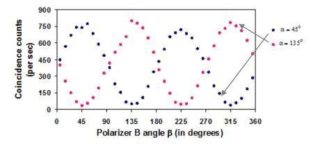
Figure 7. Polarization correlations: dependence of coincidence count on relative polarizer angle.
