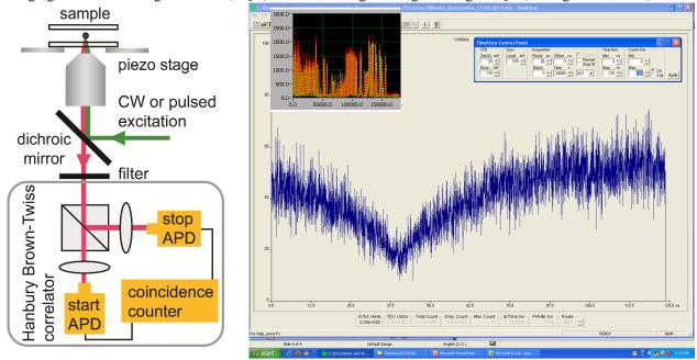
Figure 17. LEFT: Schematics of a Hanbury Brown and Twiss correlator at the ouput of a confocal fluorescence microscope (prepared by L. Bissell). RIGHT: Raw data histogram of interphoton times with a dip at zero time interval indicating photon antibunching (SPS). Fluorescence of NQD inside a gap of a bow-tie nanoantenna was studied. Insert shows a time trace of this NQD.
