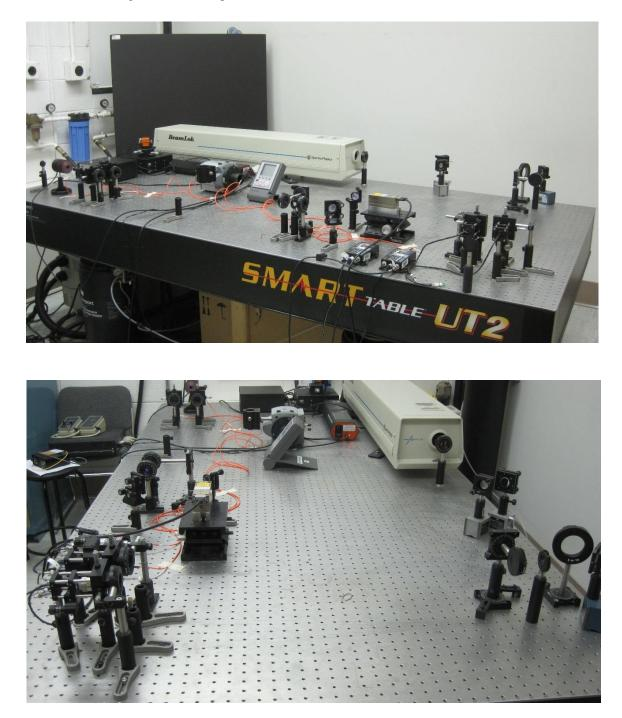
Figure 6. Two entanglement setups for the teaching labs of the Institute of Optics, University of Rochester (different views of the same optical table).
