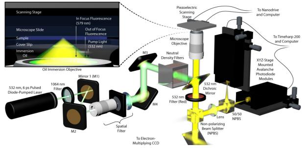
Figure 13 (prepared by R. Lopez Rios). A schematics of a confocal fluorescence microscope. Top-left inset shows oil immersion microscope objective.
