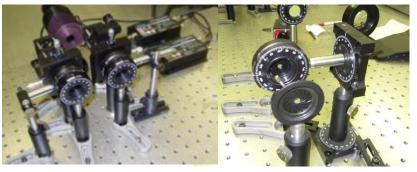
Figure 5. LEFT: Collection system with a 3-D adjustable mount with two polarizers and APD detectors. RIGHT: BBO crystal set with a 3-D rotation mounting (an iris diaphragm serves for alignment).
