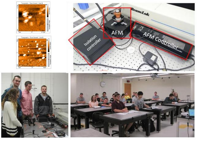
Figure 16. TOP LEFT: Raw data of AFM imaging of topography of nanodiamond clusters obtained by OPT 253 students; TOP RIGHT: A compact AFM (Easy Scan 2, Nanosurf Inc.) on a vibration isolation platform and a AFM controller. BOTTOM LEFT: Undergraduate students of a Fall 2016 OPT 253 class working on an AFM. BOTTOM RIGHT: Students of a Fall 2016 OPT 253/OPT 453 class on the lecture.
