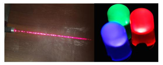
Figure 2. a) Diode laser light travelling in a straight line and visible due to scattering by the powder. b) Red, green and blue colors LED's.
