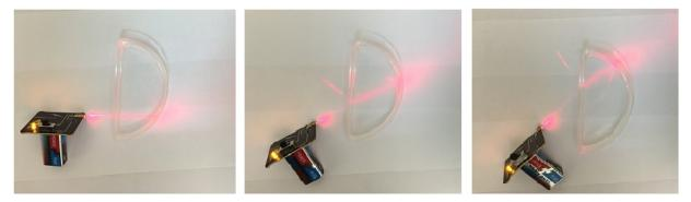
Figure 3. Reflection and refraction of light at various interfaces of a glass plate filled with water.
