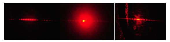
Figure 6. Diffraction pattern when laser light passes through a) Double slit b)through an obstacle and c) through a single slit.
