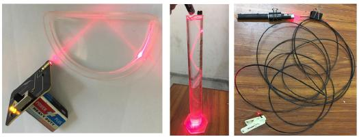
Figure 4. Total Internal Reflection of light from a) glass plate b) inside a water filled jar and c) through a fiber optics.
