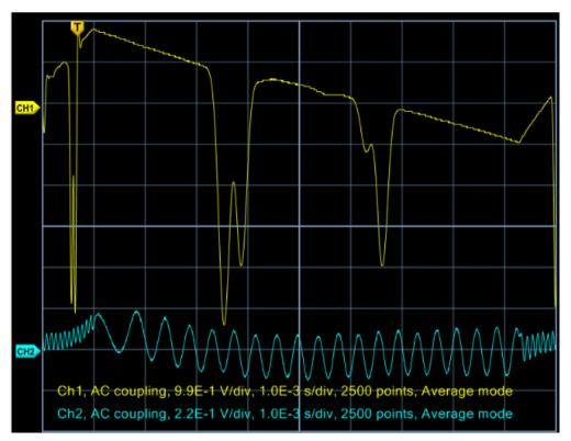
Fig. 3 Doppler limited absoprtion spectra of <sup>87</sup>Rb and resonance spectra of a solid Fabry-Perot etalon, which is used for frequency calibration.
