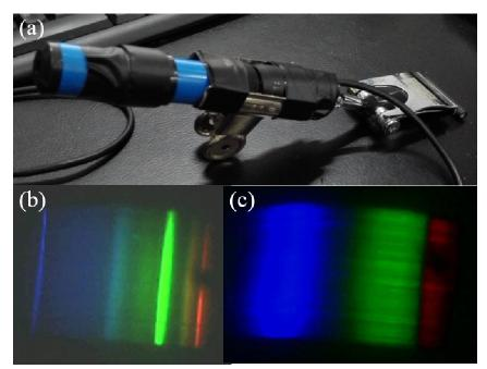
Fig. 6 (a) The picture of the simple equipment contains spectrometer and the camera. (b) and (c) are the spectroscopy of fluorescent lamps in the classroom and LED respectively.
