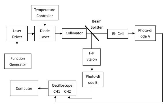
Fig.2 Schematic diagram of the diode laser spectrometer configured for Doppler limited absorption spectroscopy.
