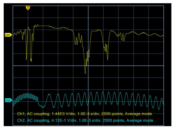
Fig. 5 Typical saturated absorption spectrum of Rubidium atom.
