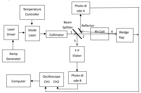
Fig. 4 Schematic diagram of the saturated absorption spectrometer.
