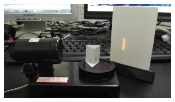
Fig. 7 The prism splits the light from the halogen lamp.
