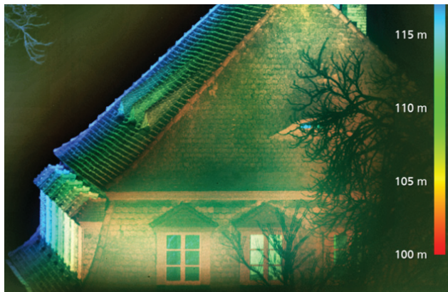
Fig. 8 Color-coded overlay of the distance dependent recording of a building with the SWIR gated viewing system.
