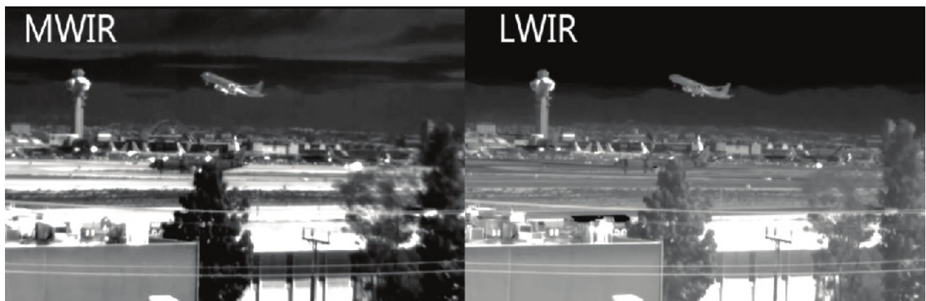
Fig. 5 MWIR and LWIR images acquired with a 1280 \times 720 format SLS array with 12 \mu\text{m} pixels dual band MW/LW FPA fabricated on VISTA. The image was captured at 80 K and f/4.
