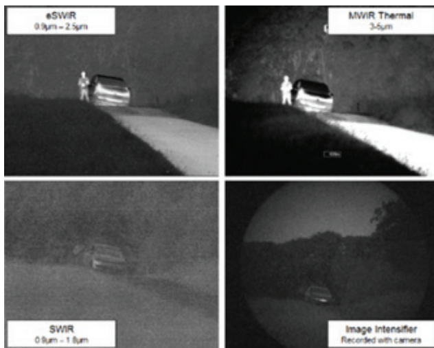
Fig. 2 Comparison of eSWIR, SWIR, MWIR 640 x 512/15 MCT FPAs with I 2 .
