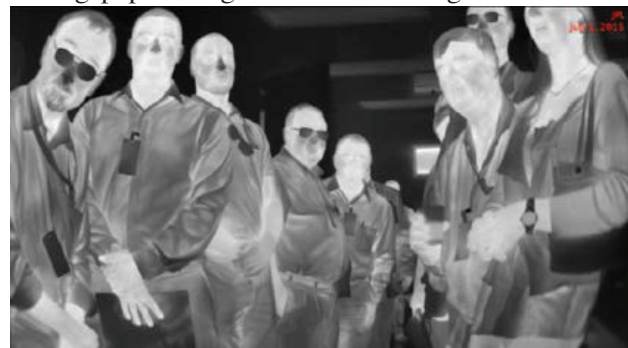
Fig. 3 Image taking from an 11 \mu\text{m} cutoff T2SL barrier infrared detector FPA with 99.4 % operability in a 1280 x 720 format.
