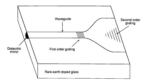
Fig. 2. Rare-earth-doped glass integrated optical symmetric beam surface emitting laser.
