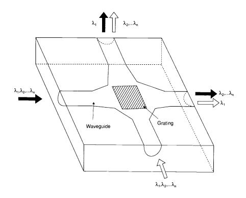
Fig. 3. Integrated optical narrow-band wavelength division multi/demultiplexer.<sup>9</sup>
