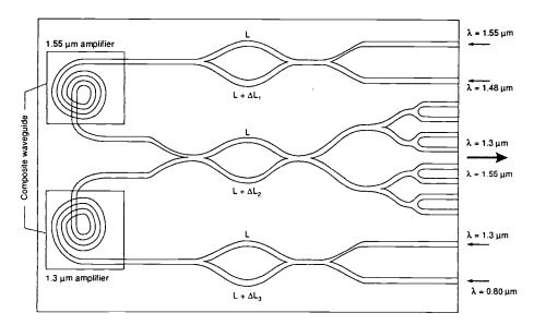
Fig. 1. 1.3  $\mu$ m/1.55  $\mu$ m glass integrated optical amplifier/splitter circuit.<sup>2</sup> The composite waveguides can be achieved using rare-earth-doped sol-gel glasses.
