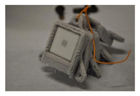
Photo 1. BiSon64-ET sunsensor housings heating up after liquid nitrogen dipping.
