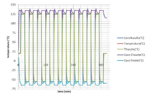
Figure 1. Thermal shock testing profile
