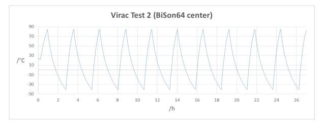
Figure 3. Typical thermal cycling profile used for BiSon64 sunsensors.
