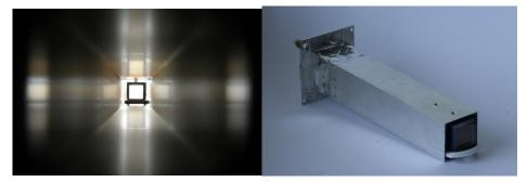
**Fig. 1** The Mini 2D LE objective with focal length of 250 mm suitable for application in cube and picosatellites. The inside view of the Mini 2D LE module (right).
