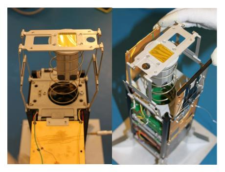
Fig. 3 The Miniature 1D LE telescope on nanosatellite VZLUSAT1..
