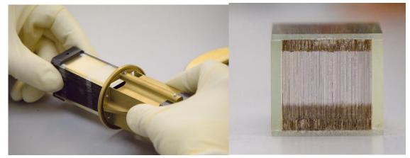
Fig. 4 The Miniature 1D LE optics for the nanosatellite VZLUSAT1..
