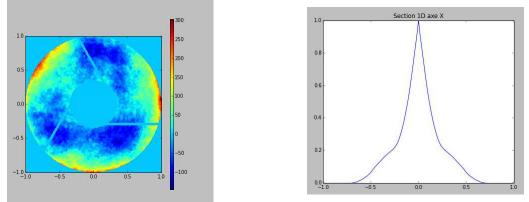
Fig 2 WFE map (left) and corresponding MTF(right)
