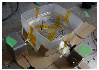
Fig.8. A fixed 3 dB-coupler by using an epoxy resin and connected PD for in-loop and out-of-loop
