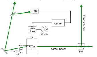
Fig.11. The experimental setup of intensity stabilization at 200 kHz. AOM: accost-optical modulator, PBS: polarized beam splitter Proc. of SPIE Vol. 10562 105620H-6
