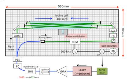
**Fig.2.** Schematic diagram of I<sub>2</sub>-stabilized laser YDFA; Yb-doped fiber amplifier, SHG; second harmonics generation Proc. of SPIE Vol. 10562 105620H-3
