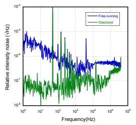
**Fig.12.** Relative intensity noise, which is controlled by AOM (evaluated by error signal) blue trace indicates free-running state and green trace indicates stabilized.
