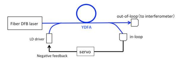
Fig.7. Schematic diagram of the intensity stabilization
