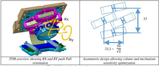
Fig. 4. BSA mechanism architecture description
