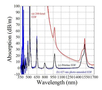
Fig. 3 RIA spectra of (a) 200-krad γ-irradiated EDF, (b) 427-nm photo-annealed EDF, and (c) the pristine EDF.
