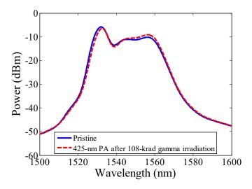
Fig. 4 Optical spectra of the FLS using (1) the pristine EDF (blue solid curve) and (2) the 425-nm photoannealed EDF after 108-krad gamma irradiation (red dashed curve)
