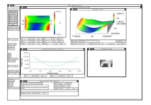
Figure 5: Slit planarity in the UV–VIS slit assembly.
