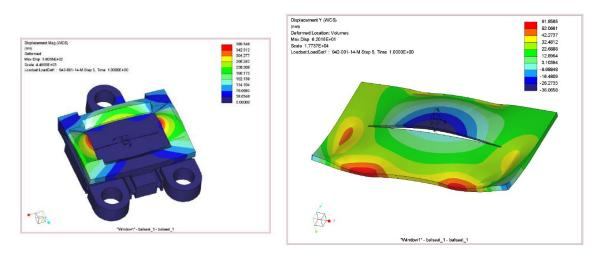
Figure 4: Finite element analyses of deformations, Left: frame. Right: slit. Proc. of SPIE Vol. 10562 105624M-5
