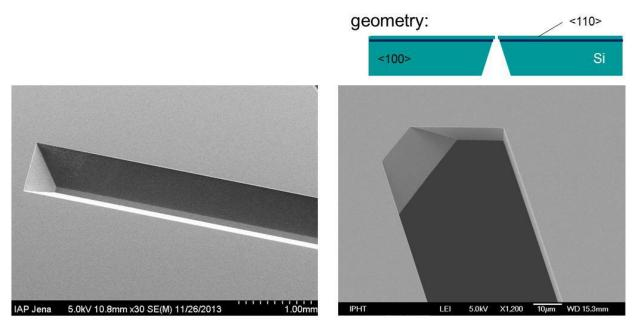
*Figure 1*: Slit manufactured in a <100>/<110> SOI wafer. Left: substrate (rear) side before removal of the SiO<sub>2</sub> etch stop between substrate and device layer. Right: slit (front) side in the device layer.
