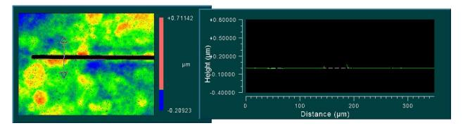
*Figure 2:* White light interferometric characterization of slit planarity after structuring. The image was taken on an area of approximately  $1200 \ \mu m \ x \ 800 \ \mu m$  near the end of the slit. The cross section of the height profile shows no structuring-induced surface deformation (except of a measurement artefact near the slit edge).
