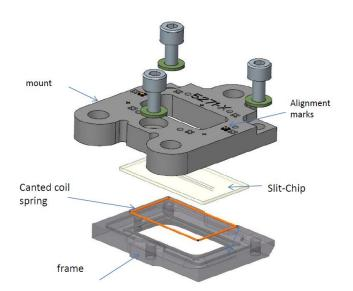
Figure 3: Components of the NIR slit assembly
