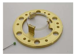
Fig. 10. Assembled lens by means of Solderjet used as representative prototype of the one used in ATLID Mission.
