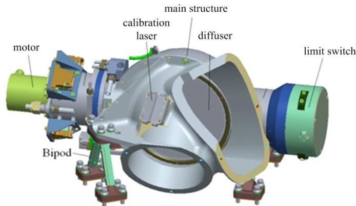
**Fig. 7.** Optic-Structure of the calibration unit
