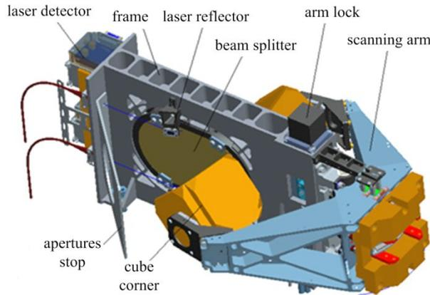
**Fig. 5.** Optic-Structure of the interferometer
