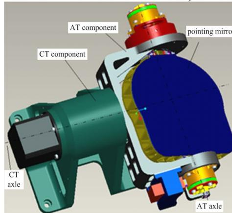
**Fig. 6.** Optic-Structure of the pointing mirror mechanism
