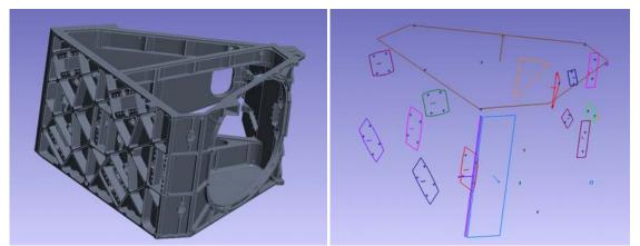
**Fig. 5** The housing structure of the primary telescope. On the left is the CAD image, on the right is the representation in the CS Engine with plane and borehole features.
