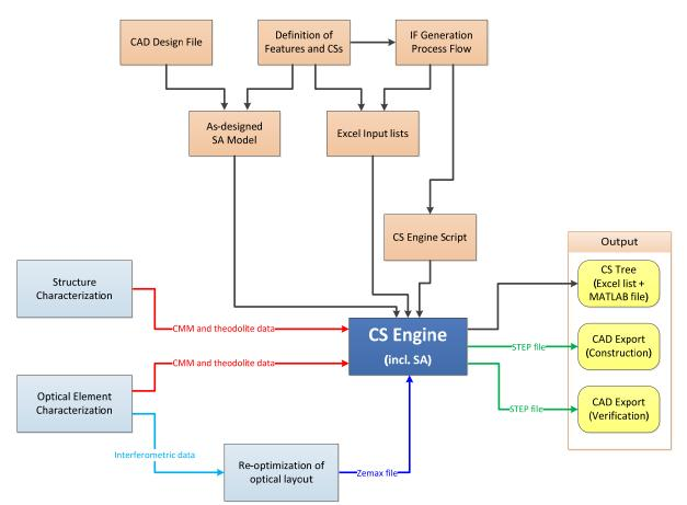
Fig. 3 The different inputs and outputs for the CS Engine during the IF generation process
