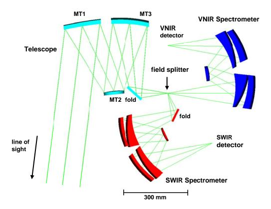
Fig. 1 A sketch of the three optical subsystems: telescope, VNIR spectrometer and SWIR spectrometer
