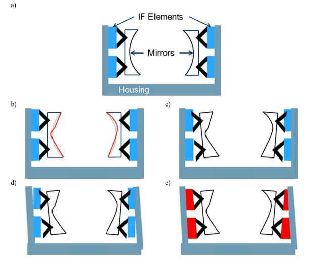
Fig. 2 A simplified sketch of the IF generation process. The design status is shown in a). Subplot b) depicts the actual surface form of the mirrors, which are compensated by adjusting the mirror positions (c). The as-built status of the housing is updated in d). The red IF elements of e) are the result of the IF generation process and place the mirrors at the intended position
