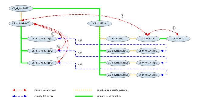
**Fig. 4** The excerpt of the IF generation flow for the telescope primary mirror (MT1) shows the hierarchical structure of the coordinate systems. The red and blue arrows indicate information from measurements and logical connections, which is used to update the CS tree from the design status to the as-built status in the order of the labelling numbers. Updated transformations are shown in green.
