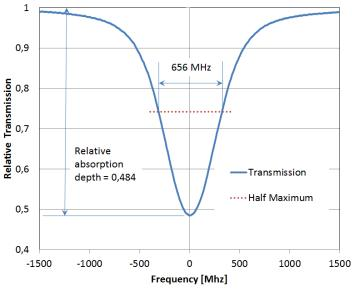
Fig. 7 : FWHM and relative transmission of a fully-integrated GCS
