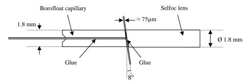
Fig. 3 : Collimator design
