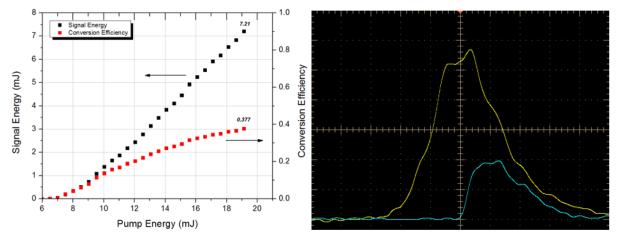
**Fig. 5.** Energy output for the VBG OPO (left); Oscilloscope trace of the depleted pump (yellow) and signal output (blue) (right).
