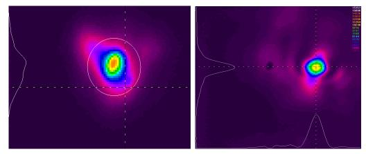
Fig. 2. Spatial profiles of the input pump beam (left) and seed beam (right).
