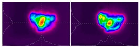
Fig. 8. Spatial profile of the amplified 2  $\mu$ m output, with crystal length L = 12 mm (left) and L = 12+7 mm (right).
