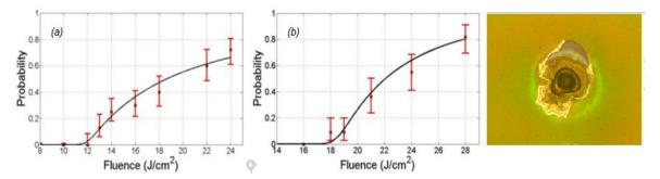
**Fig. 4.** Probability damage curve for uncoated KTP (a); Probability damage curve for AR-coated RKTP with associated damage site.
