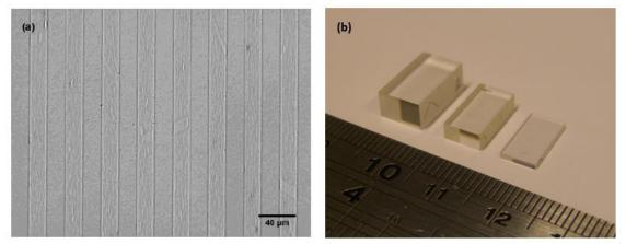
Fig. 3. Domain structures in RKTP (a); 5 mm RKTP crystal used in the experiment (b). Proc. of SPIE Vol. 10562 105620L-3
