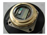
Figure 3: NEPTUNE VISIR – TEC (0.4  $\mu$ m – 2.2  $\mu$ m)
