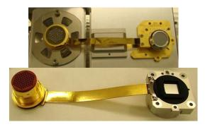
Figure 5: FCI detector (MTG FCI IR3) (top) and IRS detector (bottom)
