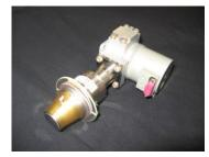
Figure 2: MARS MW IDDCA integrated in NOMAD instrument
