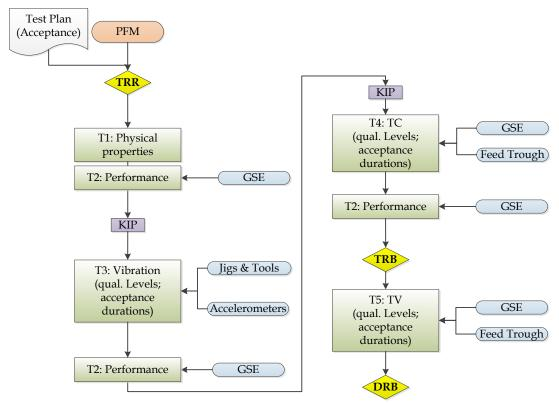
Fig. 6. CaSSIS Telescope Assembly Test Flow
