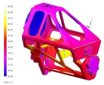
Fig. 4. CaSSIS Telescope operational Cold Case
