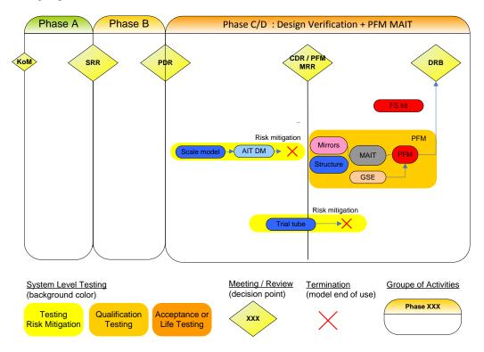
Fig. 5. CaSSIS Telescope Assembly Models Flow
