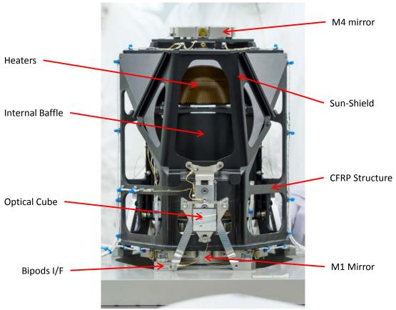
Fig. 1. CaSSIS Telescope Assembly
