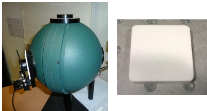
Fig. 5. Integrating Sphere and White Lambertian Spectralon
