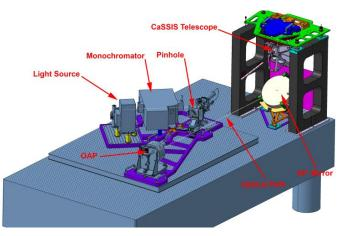
**Fig.** 9 OGSE used to integrate the detector and to test the optical performances of CaSSIS. The collimated beam obtained with an 147 mm-diameter Off Axis Parabola (OAP) and a 10  $\mu$ m pinhole and illuminated with either white (Quartz Tungsten Halogen) or monochromatic (10 nm FWHM bandpass) light. The CaSSIS telescope optical axis vertical via the 45 deg mirror to mitigate the effects of Earth gravity.
