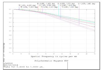
**Fig.** 7 Simulated (Zemax code) polychromatic MTF (range 400-1000nm) over the full CaSSIS FoV (1.336°x0.887°) corresponding to a 20.48 mm x 13.56 mm area on the image plane of the detector.
