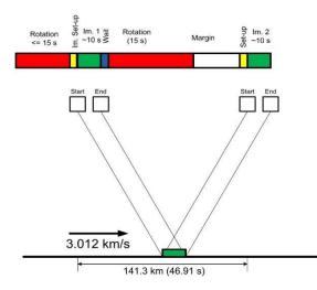
Fig. 1 Cassis telescope stereo colour observation approach
