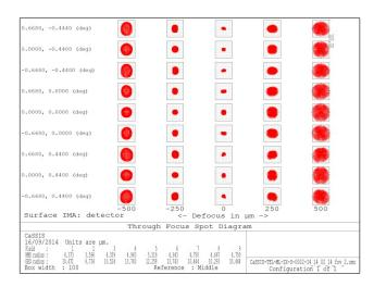
**Fig.** 8 Simulated Through focus  $\pm$  250 micron at 632 nm on detector image wrt the best focus position. (via Zemax code) and the obtained RMS spot diagrams over the full CaSSIS FoV (1.336°x0.887°) corresponding to a 20.48 mm x 13.56 mm area on the image plane of the detector. The focused spot is collected in 2x2 pixel (20 micron x 20 micron)
