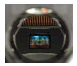
**Fig 4** Picture of the filter assembly integrated on the FPA. The FPA was illuminated by UV light to check for contamination by dust. The filter on the left of the picture is PAN, reflecting blue light and the filter on the right is BLU reflecting red and orange light. In between, the RED and NIR filters both reflect all visible light and appear like mirrors. In right side how the filters of the FPA appear through the Entrance pupil of the telescope
