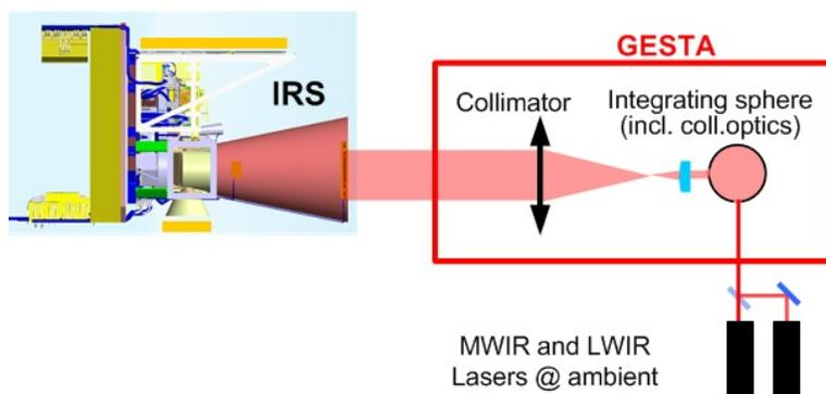
Fig. 4 ILS measurement set-up
