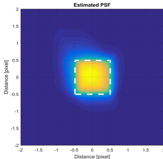
Fig. 9 Non-symmetric PSF of one pixel
