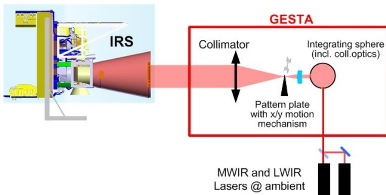
Fig. 11 Overview Straylight Test with Laser
