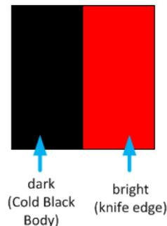
Fig. 7 Knife Edge’s plate (black: cold blackbody, red: heated KE)
