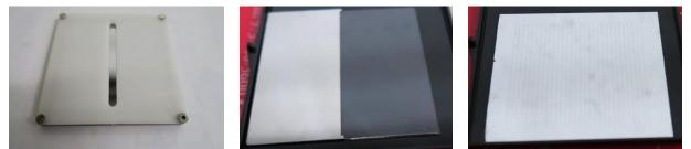
Fig. 6. Different objects that will be placed at the entrance of CSL Offner relay. (Left) 7.5µm wide slit for alignment and MTF. (Center) Knife-edge for the straylight measurement. (Right) Array of 50µm wide slits for keystone measurement.
