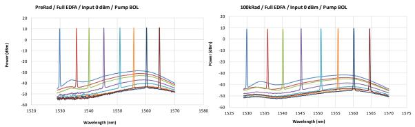
Fig. 2. Amplified signal OSA traces (left) pre-irradiation (right) post-irradiation 100 krad
