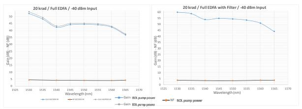
**Fig. 4.** Post-irradiation gain and noise figure vs. wavelength for the pre-amplifier at -40 dBm input. Results are shown for BOL pump power, EOL pump power: (left) with no noise management (right) with noise management.
