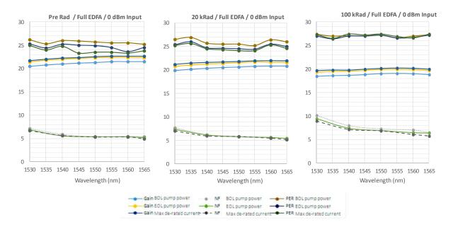
**Fig. 1.** Gain, noise figure and PER vs. wavelength for the PM EDFA using 0 dBm input. (left) pre-irradiation, (middle) post 20 krad and (right) post 100krad TID. Results are shown for BOL pump power, EOL pump power and pump power at maximum de-rated pump driving current
