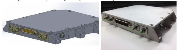
Fig. 6. EM fiber amplifier unit: (left) CAD drawing, (right) assembled unit.
