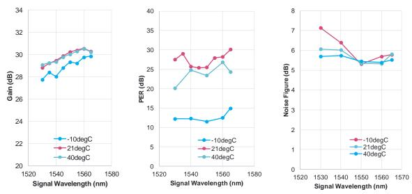
**Fig. 7.** PM-booster EM-EDFA performance over qualification temperature range: (left) gain, (middle) PER, (right) NF.
