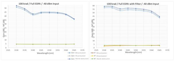
**Fig. 5.** Post-irradiation gain and noise figure vs. wavelength for the pre-amplifier at -40 dBm input. Results are shown for BOL pump power EOL pump power and pump power at maximum de-rated driving current of the pump diode: (left) with no noise management (right) with noise management.
