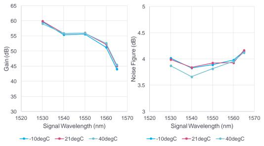
**Fig. 8.** Pre-amplifier EM-EDFA performance over qualification temperature range: (left) gain, (middle) PER, (right) NF.
