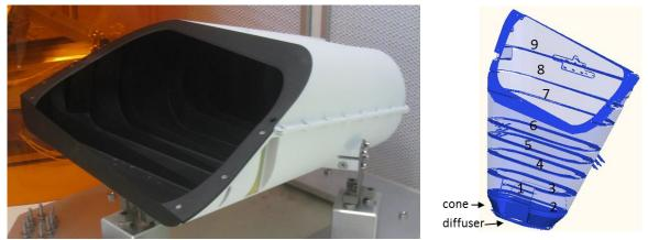
Figure 2: Picture and sketch of the sun baffle.
