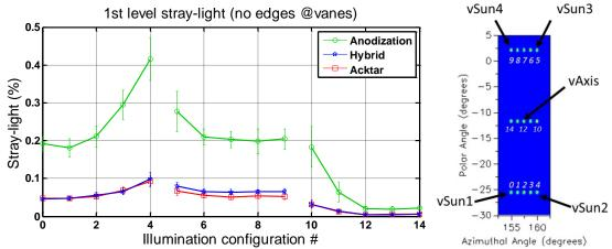
Figure 5: (left) 1<sup>st</sup> level stray-light @diffuser level, due to the direct sun illumination on the baffle, excluding the effect of vanes edges. (Right) Illumination configuration (UVN global reference frame)
