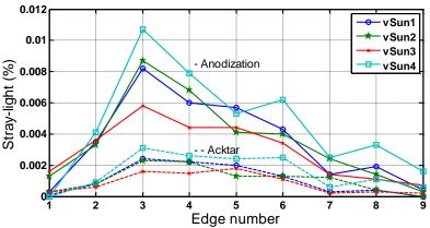
Figure 6: 1<sup>st</sup> level stray-light @diffuser level, due only to direct illumination on the vanes edges. Continuous and dotted curves are respectively the case of black anodization and acktar coating.
