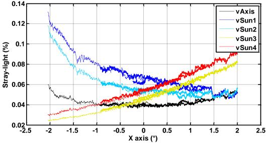
Figure 10: Experimental characterization of the stray-light for different configurations of sun illumination.
