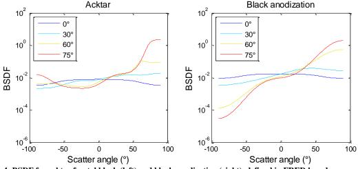
Figure 4: BSDF for acktar fractal black (left) and black anodization (right), defined in FRED based on experimental datas
