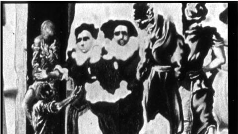
**Fig. 10.** Still-image (512x1024) produced by projecting a diapositive onto the sensor and using a flushintegrate-flush sequence with 20ms integration time. The black rectangular shapes on the left, top and right of the picture are caused by the use of metal shields, one can see two 4x4 pixels pinholes in the right black rectangle.
