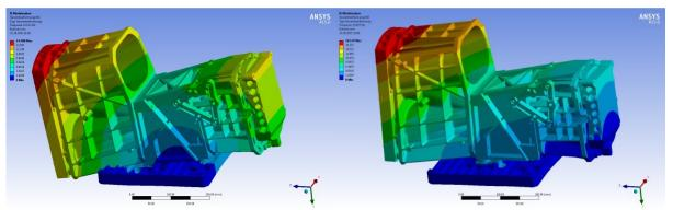
**Fig. 11.** Vibrational Eigenmodes of the opto-mechanical system. The fundamental mode at 123 Hz is shown in the left, while the second mode at 235 Hz is shown in the right picture.
