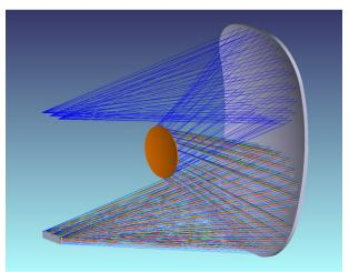
Fig. 3. Scheme of the Offner-type spectrometer.
