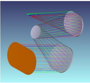
Fig. 1. Lay-out of the TMA.
