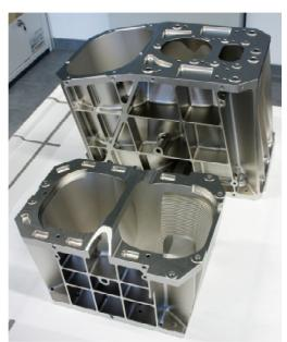
Fig. 10. TMA (top) and spectrometer (bottom) housing elements prior to coating.
