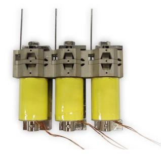
Fig. 2. A strip of 3 prototype electromagnetic actuators to be used in a deformable mirror. This strip enables a rectangular actuator grid with a minimal pitch of 18mm
