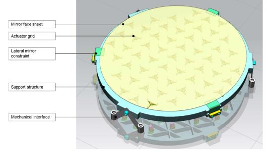
**Fig. 5.** Impression of the DM for space applications based on 57 electromagnetic actuators as shown in Figure 2. The mirror dimensions are an elliptical 610x670mm.
