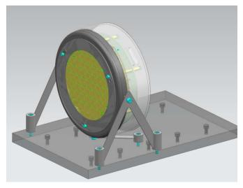
Fig. 7. Impression of the DM prototype designated for the adaptive optics correction chain breadboard.
