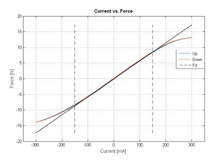
**Fig. 4.** Actuator force response for a  $\pm 300$ mA driving current (blue and red curve). The black solid line shows the linear fit over the  $\pm 150$ mA range over which the force output is  $\pm 8$ N. The linearity over this range is 99.5%, and the hysteresis is less than 1%.
