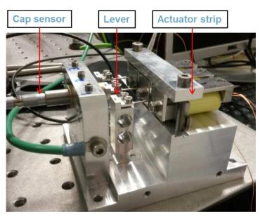
**Fig. 3**. Actuator test-rig. The actuators are pushing against a lever which stiffness is similar to the stiffness of the face sheet in the DM. The displacement of the lever is measured by a cap-sensor. The stiffness of the levers are calibrated via a force-probe
