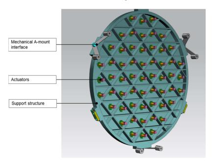
Fig. 6. Backside view of the DM for space applications. Proc. of SPIE Vol. 10562 1056230-6
