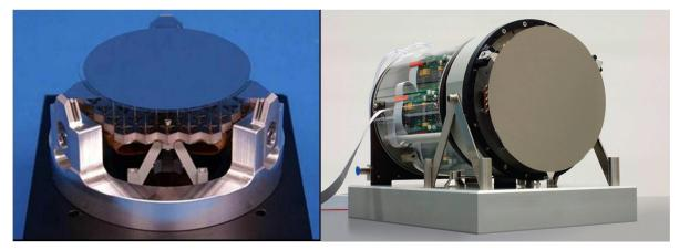
Fig. 1. First deformable mirror prototypes of TNO, containing 61 (left), and 427 actuators right [5].
