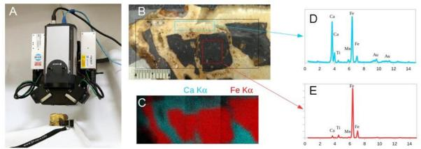
Fig. 4: MapX-II prototype. A) instrument in position to analyze a rock sample. B) Optical image of sample composed of breccia fragments and light-toned cement (scale is in mm). C) Fe  $K\alpha$  / Ca  $K\alpha$  map obtained by tiling 3 analyses of 1000s integration. D&E) XRF spectra of two ROIs
