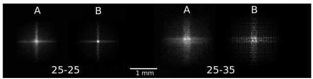
Fig. 6: Comparison of PSF data collected at SSRL BL2-3 (A) and obtained by ray tracing simulations (B) at a nominal CCD-MPO distance of 25 mm and 7.5 keV energy (Ni K $\alpha$ ). Left: sample in focus (25-25); Right: sample out of focus by 10mm (25-35) resulting in a loss of resolution of ~100  $\mu$ m.
