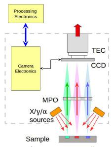
Fig. 1: Principal components of MapX:  $X/\gamma/\alpha$  source illuminates the surface of the sample. fluoresced X-rays pass through a Multi Pore Optic (MPO) and are focused on the Charge Couple Device (CCD) detector, in direct detection, cooled by a multistage Peltier Thermo Electric Cooler (TEC)
