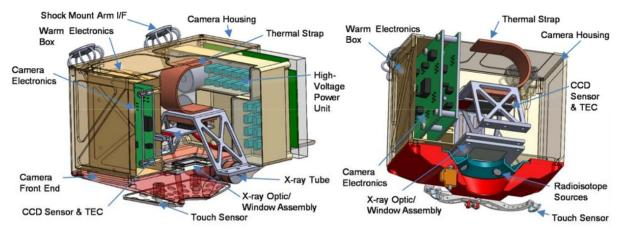
Fig. 3: Preliminary designs of two flight configurations of the MapX Arm Unit: Left:X-ray tube source based design, Right: more compact radioisotope based design.
