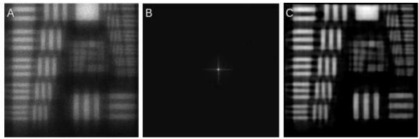
Fig. 7: MapX PSF Deconvolution Example. A) Original image. Chromium  $K\alpha$  X-rays (5.4 keV) taken with MapX-II (MPO-CCD = MPO-Target = 50 mm). The resolution of this image is estimated to be 200  $\mu$ m. B) Point Spread Function measured at the Stanford synchrotron (FWHM ~165  $\mu$ m). C) AIDA deconvolution with automatized cost function parameters (resolution ~135  $\mu$ m).
