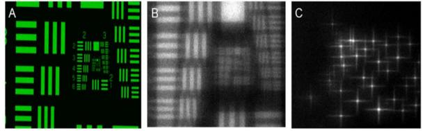
Fig. 5: Resolution test of MapX-II. USAF 1951 imaging standard, Cr on Glass. A) Cr image obtained in a commercial EDAX Orbis PC instrument with a 30 µm polycapillary optic (~80 µm resolution). B) Raw Cr map measured with the MapX-II instrument. Resolution is decreased as a result of the MPO lens PSF. C) Raw Fe map of 60 µm Fe particles with the MapX-II instrument. The Fe particles that appear as crosses, in which photon intensity is spread away from the source particles in x and y directions.
