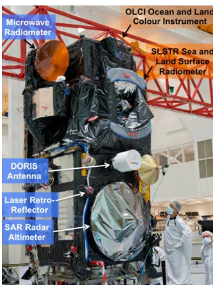
Fig. 1. The Sentinel-3A satellite fully equipped during on-ground testing at Thales Alenia Space, France, in December 2014.
