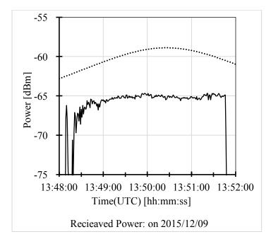
**Fig. 5.** The detected and estimated received power during the experiment at NICT Kogani OGS. The receive timing is 13:48:00 to 13:52:00 9th December, 2015, in UTC. (Solid: detected, Dotted: estimated, without the loss of atmosphere)
