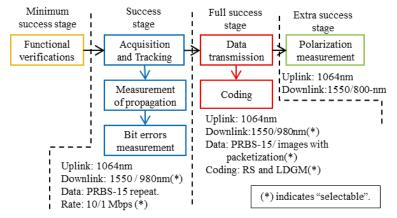
Fig. 3. The experimental plan chart and success criteria of SOTA project
