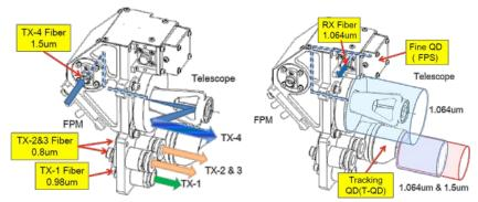
Fig. 2. The optical paths of SOTA optical part, the transmitter system (left), the receiver system (right)
