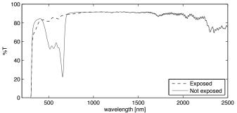
Fig. 2. UV-vis-NIR spectra of the Bayfol<sup>®</sup> TP16 photopolymeric material before (solid line) and after photobleaching (dashed line).
