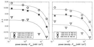
**Fig. 3.**  $\Delta n$  as function of the mean value of the intensity of the two writing arms. The total dose was kept constant at 42 mJ/cm<sup>2</sup> (referred to double beam writing process).
