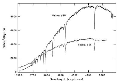
**Fig. 4.** Comparison of photometric-standard stars' spectra SP0305+261. Total system throughput of the NOT telescope with Grism #16 and Grism #18. Slitwidth used in the observations is 10.0 arcsec.
