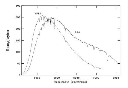
**Fig. 6.** Comparison of photometric-standard stars' spectra. Total system throughput of the Asiago's telescope with GRISM VPHG7 and grating GR4. Slitwidth used in the observations is 4.22 arcsec.
