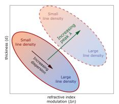
Fig. 1. Scheme reporting the general rules for designing high efficient and wideband VPHGs in the  $d - \Delta n$  space.
