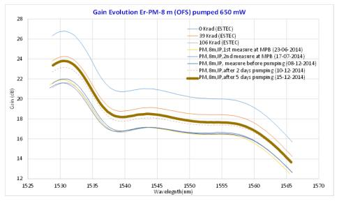
Fig. 8: Evolution of EDF-PM from OFS, Irradiated, pumped during irradiation at 650 mW Proc. of SPIE Vol. 10562 1056219-7
