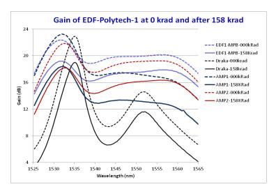
Fig. 4: Polytech-1 Gain spectra before (dashed lines) and after 158 krad the shape is kept Proc. of SPIE Vol. 10562 1056219-5
