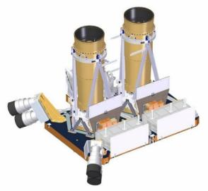
Fig. 1. 3D view of the Ingenio/SEOSAT primary payload
