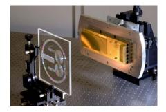
**Fig. 6.** Measurement of the mirror module in the profilometer UA3P 650H from Panasonic with a 5 μm diamond stylus at Fraunhofer IOF (left); measurement setup with multi aperture CGH for a smaller mirror module, sample from PREMIER instrument (right) [5; 8; 10; 13].
