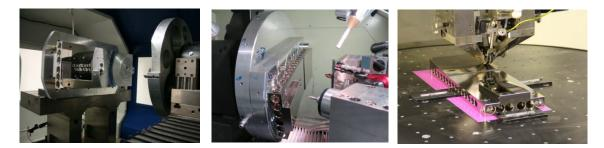
**Fig. 5.** Manufacturing steps of mirror module; left: UP fly-cutting of rear site; middle: combination of diamond turning and milling in one setup; right: MRF correction with 50 mm polishing wheel [14].
