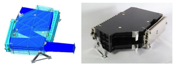
Fig. 10. CAD model of the complete telescope (left); final telescope demonstrator (right) [14].
