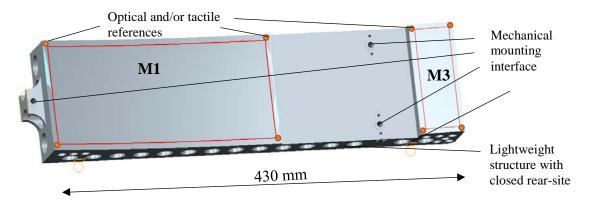
**Fig. 3.** CAD layout of the mirror module M1-M3 including the optical surfaces M1 and M3, ultra-precisely machined mounting interfaces, and reference spheres for tactile and/or interferometric metrology.
