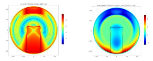
**Fig. 4.** Manufacturing analysis; left: azimuthal acceleration of the tool; right: freeform portion (equivalent to fast tool travel) for diamond turning of both optical surfaces in a single tool path for mirror module M1-M3.
