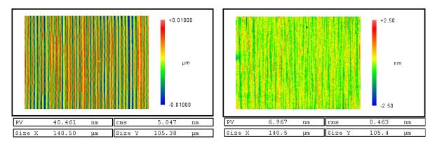
**Fig. 1.** Roughness of a metal mirror (magnification 50x; measuring range 141µm x 105µm); left: after diamond turning with typical pattern; right: after MRF polishing [8].
