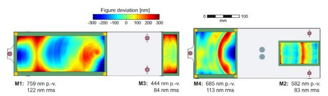
Fig. 7. Shape- and relative position deviations of the mirror modules M1-M3 (left) and M2-M4 (right) after ultra-precise diamond machining [14].
