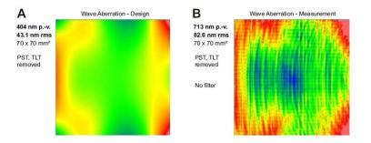
Fig. 11. Experimentally determined system wavefront of the anamorphic telescope in the central field point, A: designed wavefront 404 nm p.-v. / 43 nm rms; B: measured wavefront 713 nm p.-v. / 83 nm rms [14]. Proc. of SPIE Vol. 10562 105625T-8
