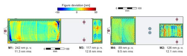
Fig. 8. Shape- and relative position deviations of the mirror modules M1-M3 and M2-M4 after MRF [14].
