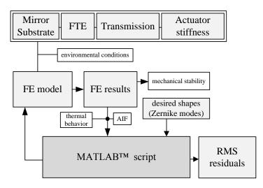
Fig. 6. Development routine of the DM design process
