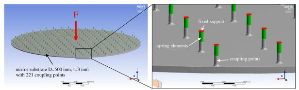
Fig. 4. Simplified FE-model. It consists of the mirror substrate, coupling points and spring elements
