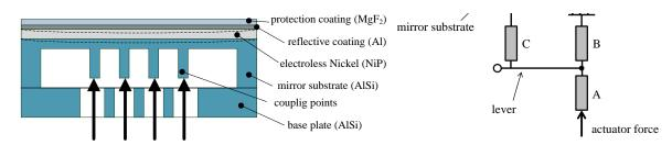
Fig. 7. Left: Semi-monolithical concept for the deformable mirror, Right: equivalent circuit of the transmission elements
