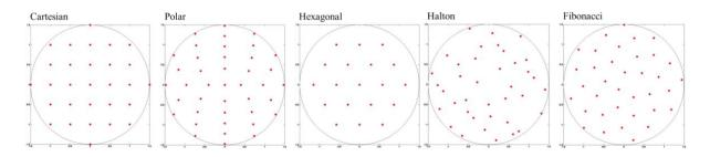
**Fig. 2.** Distribution of 36 actuators for the five analysed grid variants. The substrate is extended by the factor of 1.5 with respect to the diameter of the mirror surface. The red dots show the centers of the actuator influence
