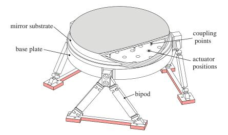
**Fig. 4.** Mounting concept for the deformable mirror with three bipod flexures in a 120-degree-arrangement. The red marked surfaces of the bipods are used to mount the DM with the HYPATIA telescope structure.
