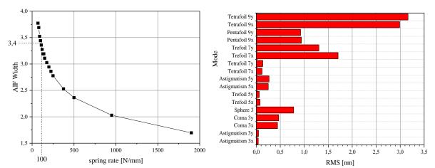
Fig. 5. Left: Width of the actuator influence function depending on the stiffness of the mirror support. Right: Residual RMS error of the desired Zernike modes with an AIF width of 3.4 Proc. of SPIE Vol. 10562 1056233-5
