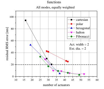
Fig. 3. The residual RMS error obtained by summing the residual RMS error of the individual Zernike modes as a function of the number of actuators for different actuator geometries
